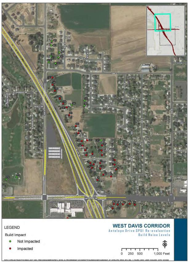
Figure 3. Build Scenario Noise Receptor Map [1 of 2]
